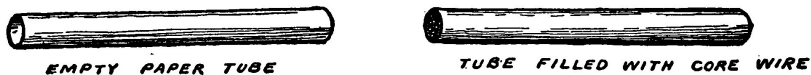
Fig. 158.—Empty Paper Tube, and Tube filled with Core Wire preparatory to winding on the Primary.
